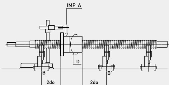
T6 : Run-out deviation of external diameter (only for nut) relative to BB' (This measurement is made according to DIN 69051 and JIS B1192)
