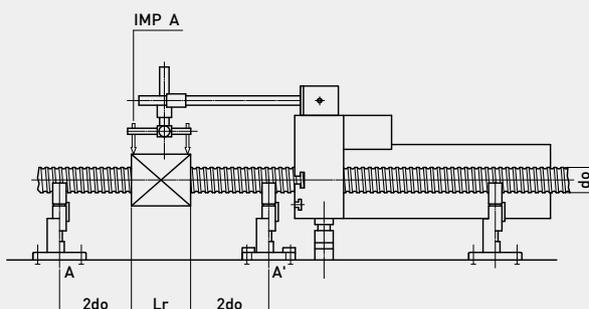
T7 : Deviation of parallelism (only for nut) relative to BB' (This measurement is made according to DIN 69051 and JIS B1192 )
