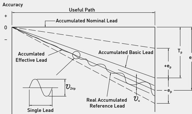
$T_p$  : Target point of accumulated lead.
