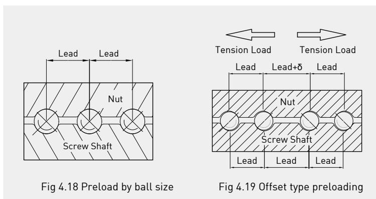
Fig 4.18 Preload by ball size
