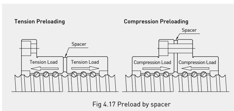
Fig 4.17 Preload by spacer
