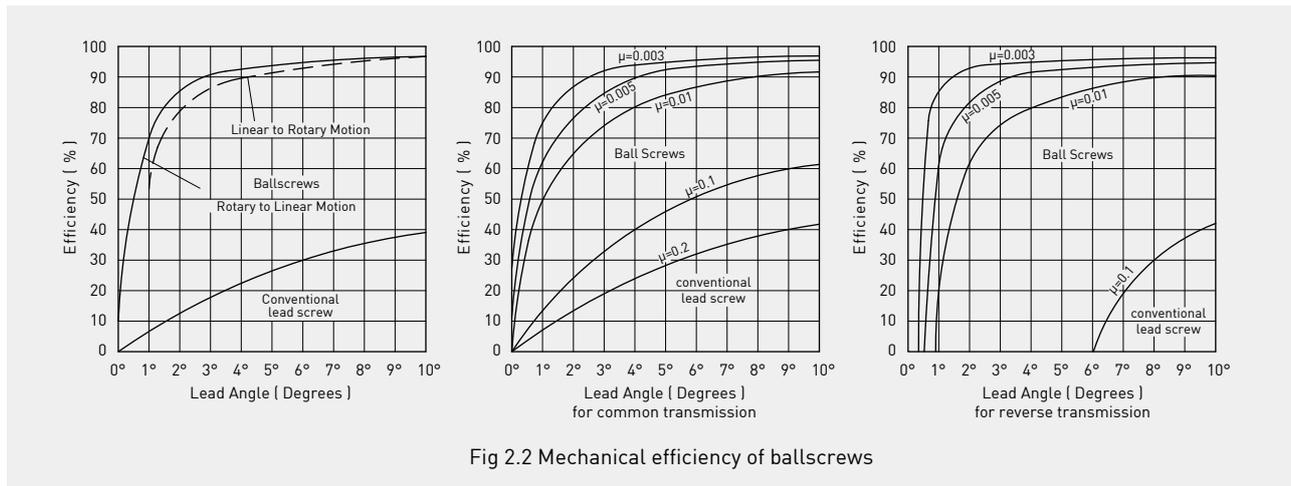
Fig 2.2 Mechanical efficiency of ballscrews
