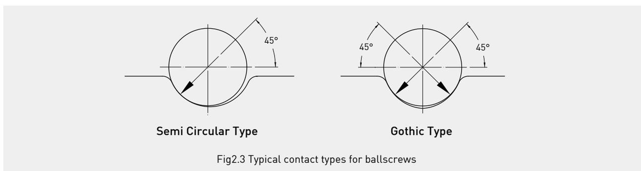
Fig2.3 Typical contact types for ballscrews
