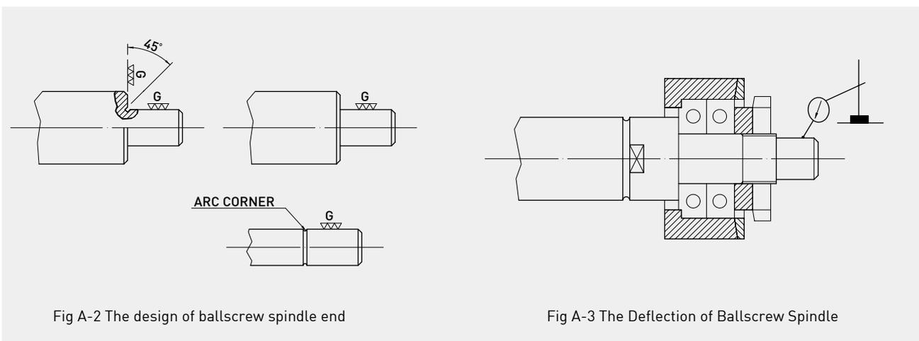
Fig A-2 The design of ballscrew spindle end
