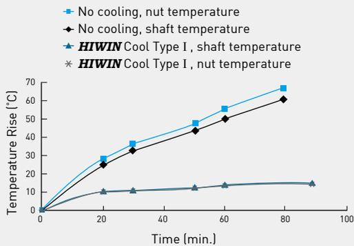
Fig. 8.5 Cool type I : Temperature rise of ballscrew
