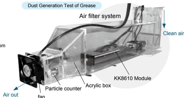
Test Condition : Air speed 2.5m/s
