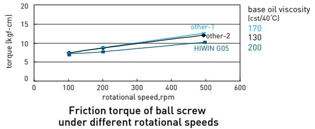
Friction torque of ball screw under different rotational speeds
