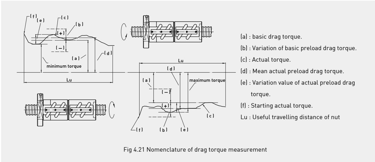
Fig 4.21 Nomenclature of drag torque measurement
