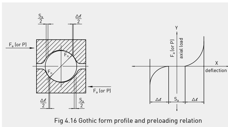
Fig 4.16 Gothic form profile and preloading relation
