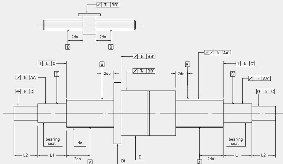
Fig 4.15 Geometrical tolerance of HIWIN precision ground ballscrew
