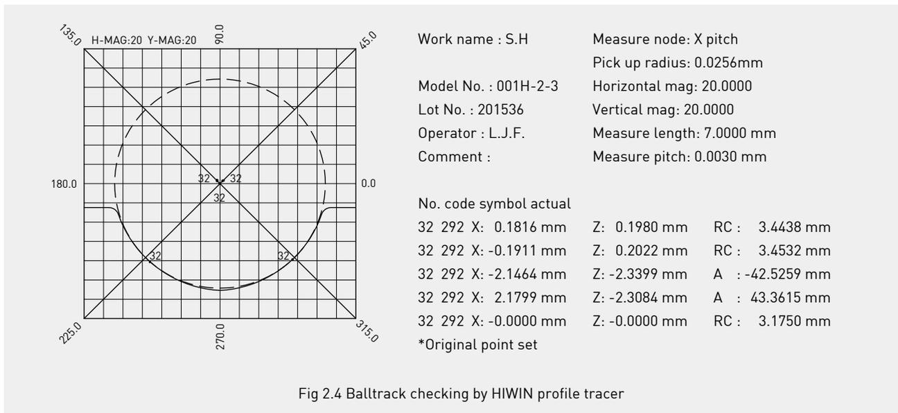
Fig 2.4 Balltrack checking by HIWIN profile tracer
