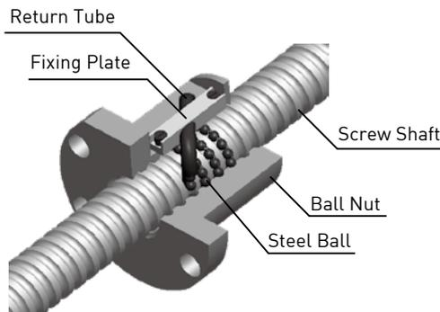
Fig. 3.1 External recirculation type nut with return tubes
