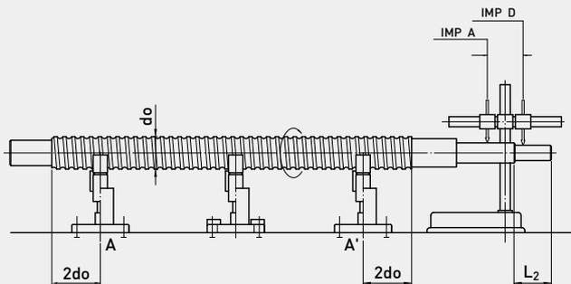
T3: Coaxial deviation relative to AA' (This measurement is made according to DIN 69051 and JIS B1192)
