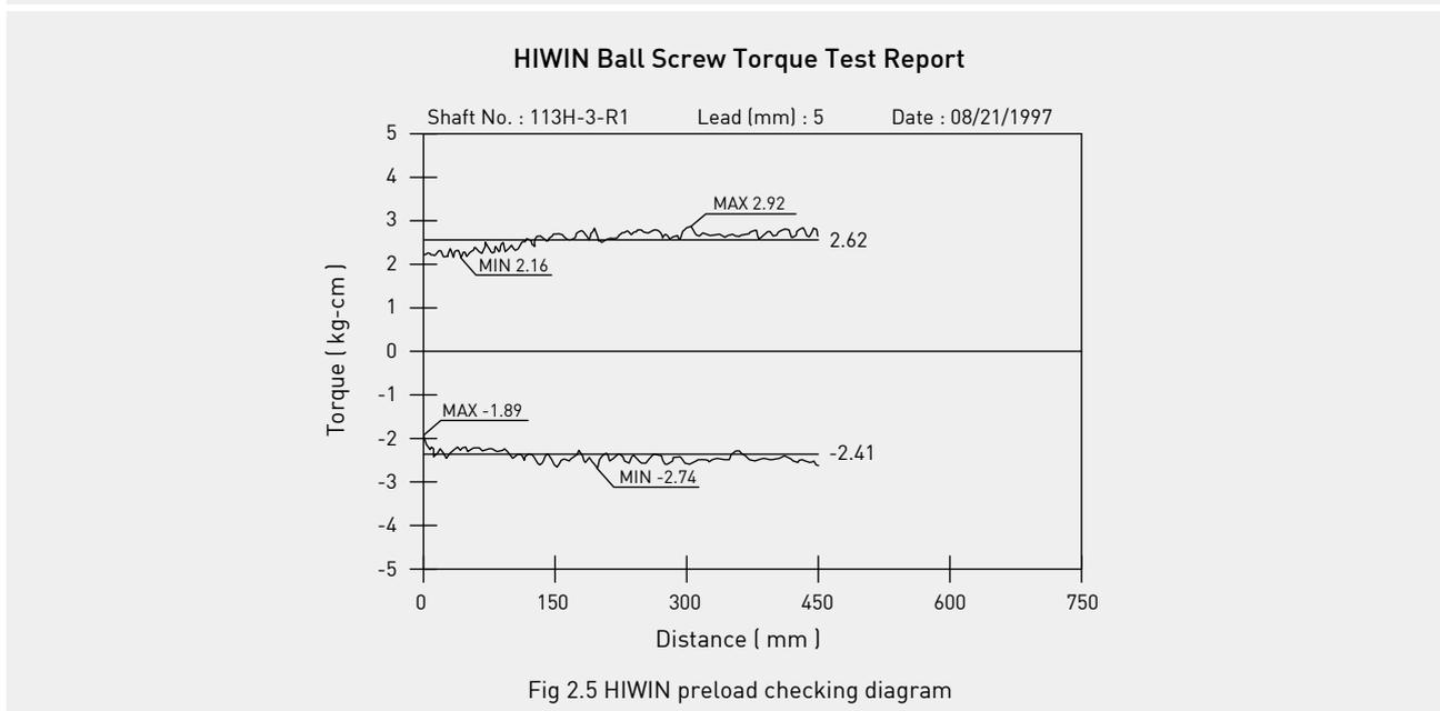
Fig 2.5 HIWIN preload checking diagram
