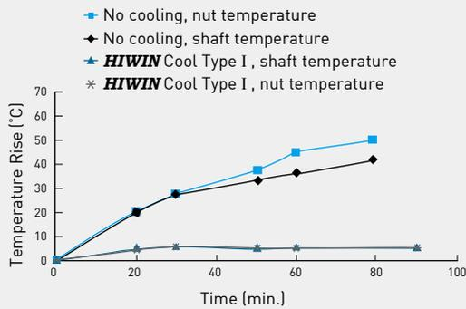
Fig. 8.4 Cool type I : Temperature rise of ballscrew
