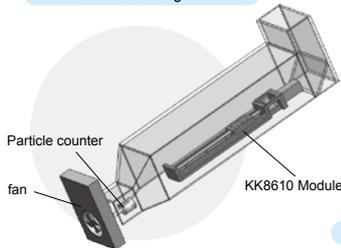
Dust Generation Test of Grease
