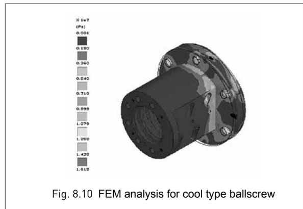
Fig. 8.10 FEM analysis for cool type ballscrew
