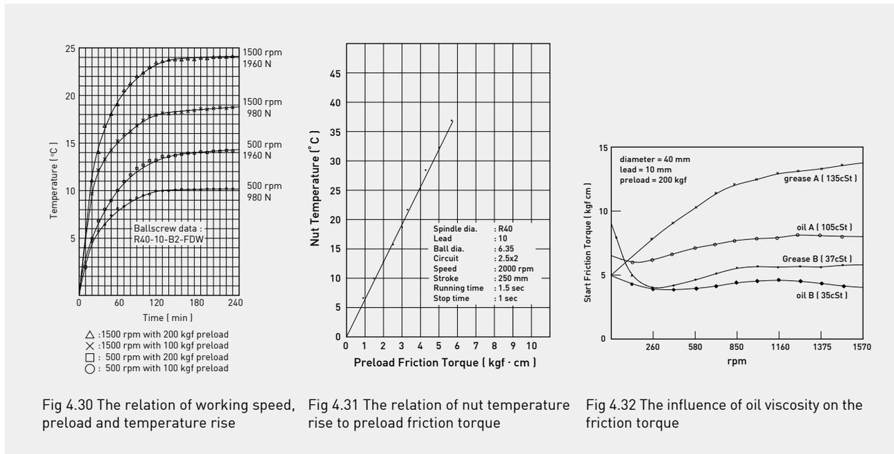
Fig 4.30 The relation of working speed, preload and temperature rise
