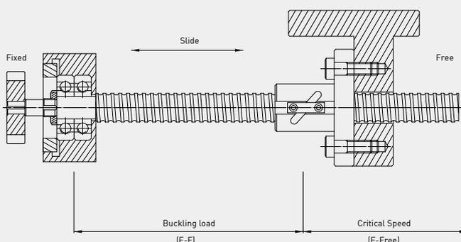
Fig 4.27 Supporting conditions for screw shaft ball nut
