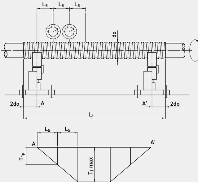
T1: True running deviation of external diameter relative to AA' (This measurement is made according to DIN 69051 and JIS B1192)
