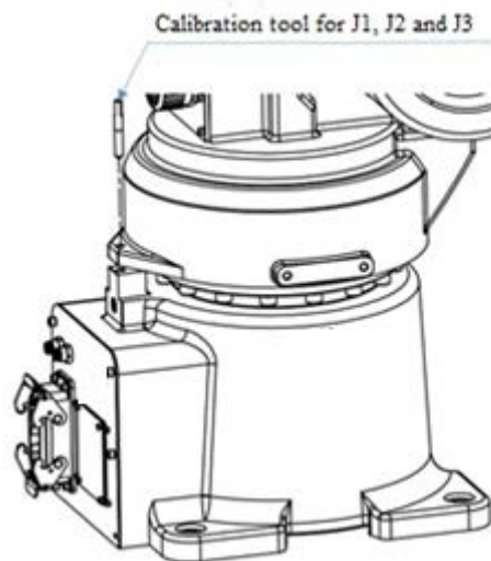
Figure 4-2 Illustration of J1-axis zero position setting
