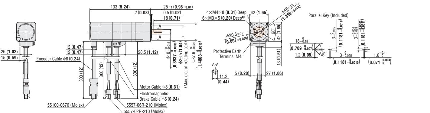
\*The position of the output shaft and the positions of the screw holes cannot be specified in a dimensions drawing, so please do not design using the screw hole dimensions of the load installation surface.
