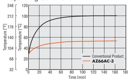
**47% Less Power Consumption than Conventional Oriental Motor Products Due to Energy-Saving Features**
