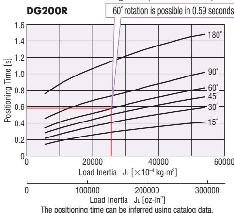
The positioning time can be inferred using catalog data.
