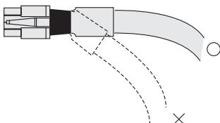
② For the bending radius, use at 6 times min. of the cable diameter.
