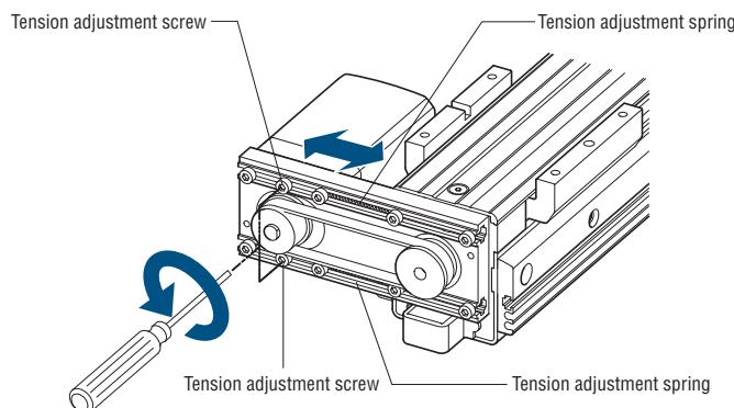
If the screw is loosened, the belt tension is adjusted to an appropriate value by the force of the spring.
