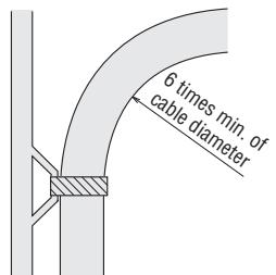
③ The cable from the motor and the accessory cable are not bending types. If the motor cable is to be bent, bend it at the flexible cable.
