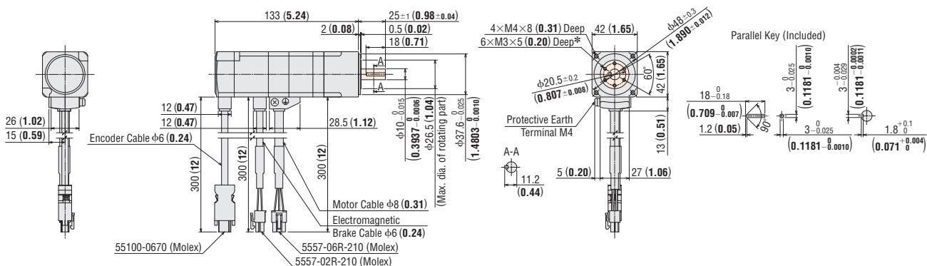
\*The position of the output shaft and the positions of the screw holes cannot be specified in a dimensions drawing, so please do not design using the screw hole dimensions of the load installation surface.
