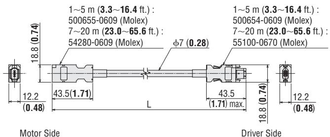
\*The length L [m (in.)] in "■ Product Line and List Price" on pages from 14 to 16 is entered where L is located in the dimensions drawing.
