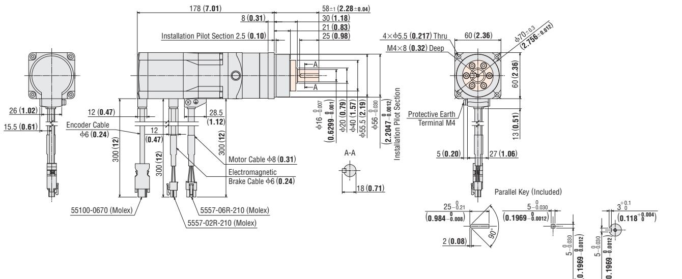
◇ HPG Geared Type with Electromagnetic Brake Flange Output Type
