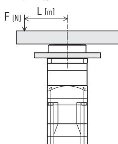
**Example 2:** An external force F1 is applied from the output flange installation surface at distance L
