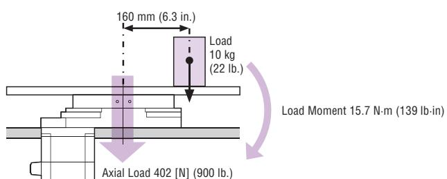
**It is possible to apply heavy loads at positions that are far from the center of the high rigidity hollow actuator table**
