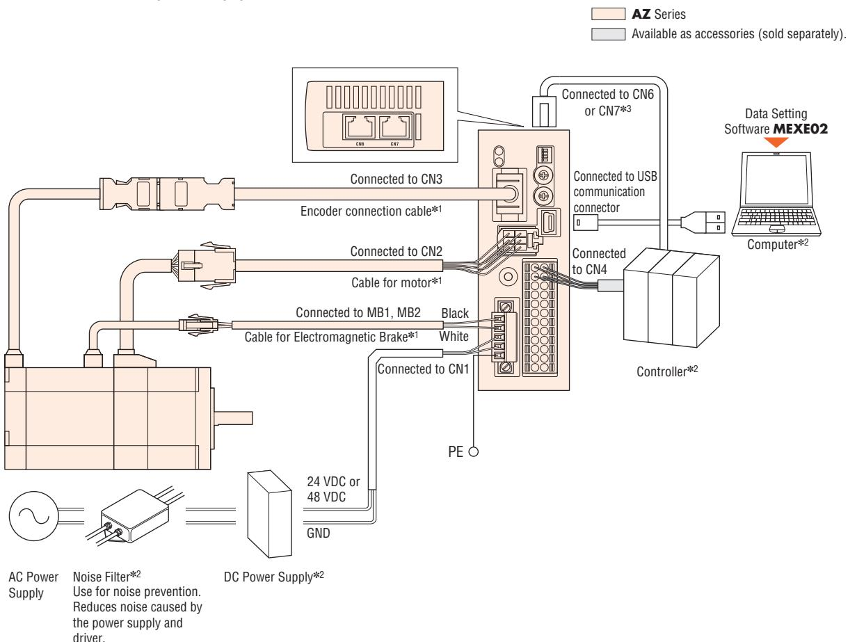
\*1 When wiring the motor and driver, keep a max. distance of 20 m (65.6 ft.).
