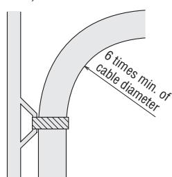
③ The cable from the motor and the accessory cable are not bending types. If the motor cable is to be bent, bend it at the flexible cable.
