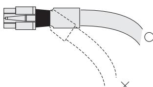
② For the bending radius, use at 6 times min. of the cable diameter.
