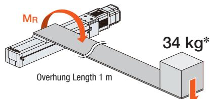
\*The load is calculated using the static permissible moment 340 N·m of the **EZS**.
