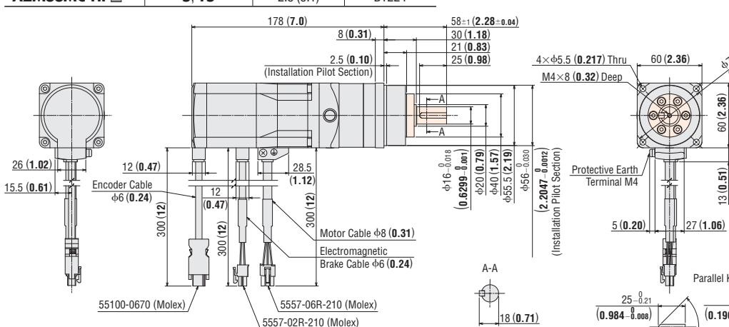
● The color ■ in the dimensions drawing indicates the rotating part.
