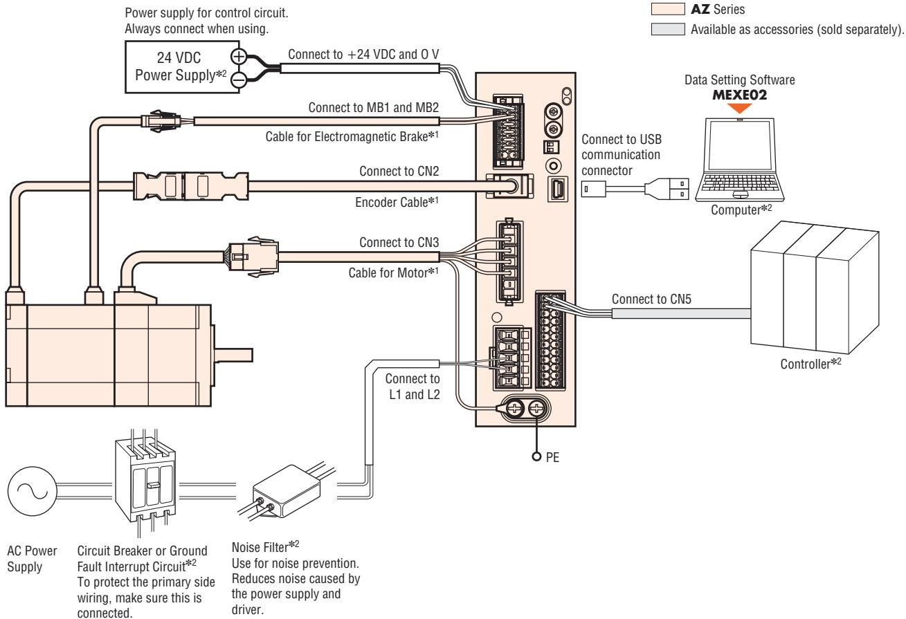
\*1 Keep the maximum wiring distance between the motor and driver to 20 m (65.6 ft.).
