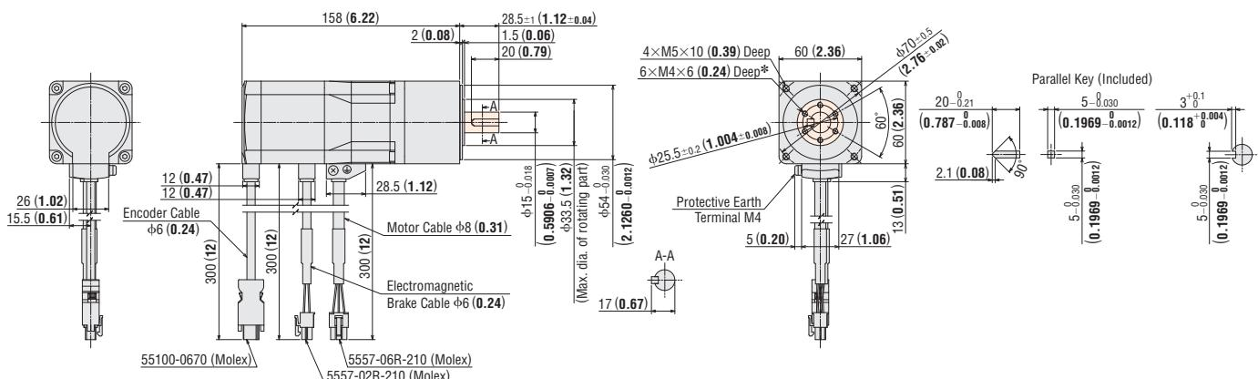
\*The position of the output shaft and the positions of the screw holes cannot be specified in a dimensions drawing, so please do not design using the screw hole dimensions of the load installation surface.
