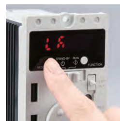
The dial operation can be locked.
