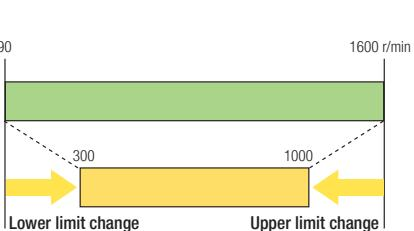
Speed range for speed setting can be limited in advance.
